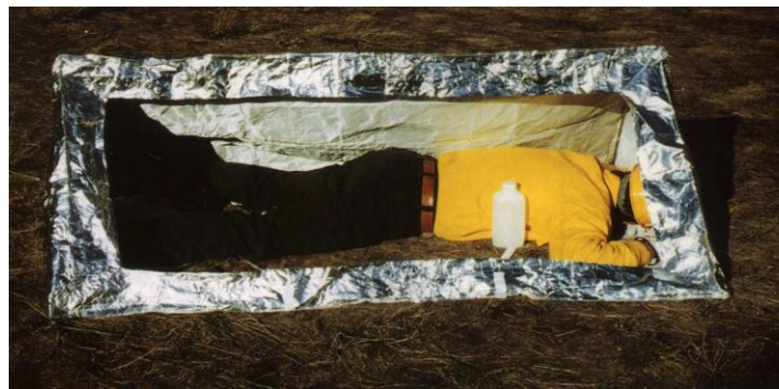
Figure 1 —The fire shelter reflects radiant heat and absorbs convective heat.
